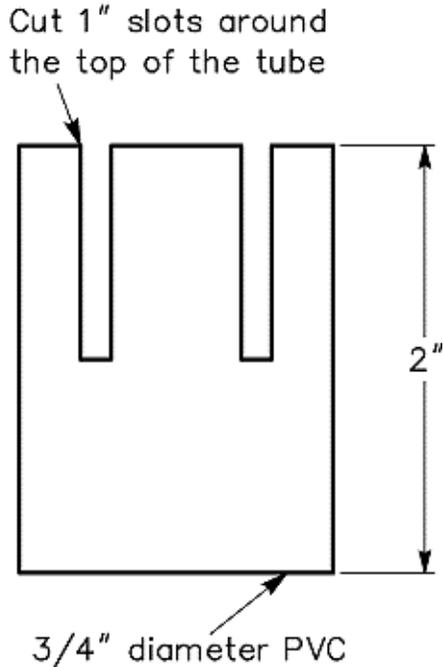
**Figure 3—Make two clamps by cutting 1-inch slots into two 2-inch long, 3/4-inch diameter PVC tubes. When you tighten the steel hose clamps around these slots, they'll apply firm pressure to the PL-259 connectors, holding the ground planes in place.**
