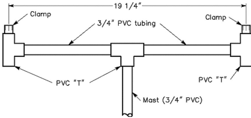
**Figure 2—Assemble the boom using  $\frac{3}{4}$ -inch diameter PVC tubing and Ts. Note that the distance is  $19\frac{1}{4}$  inches between the center of one PVC "end T" and the other.**
