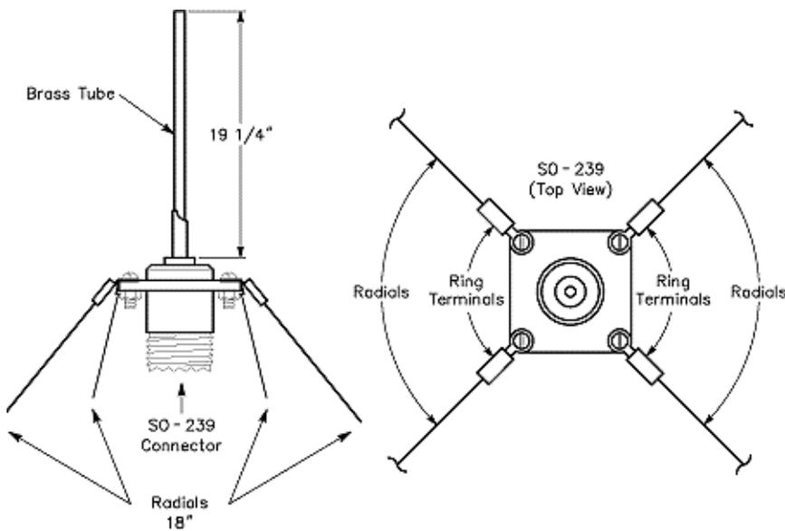
**Figure 1—First you need to build two ground plane antennas as shown. Use brass tubes for the vertical radiators and stiff copper or aluminum wire for the radials. Ring terminals, screws and nuts secure the radials to the SO-239 chassis connectors.**
