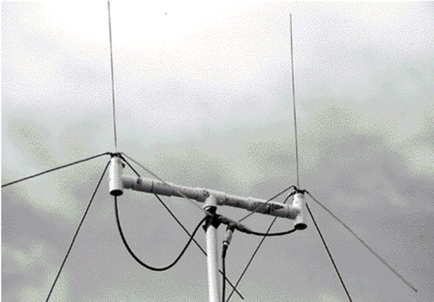
**Figure 6—The assembled phased array antenna. Note how the two phasing lines reach the ground planes through the bottoms of the PVC T sections. The entire array radiates in the direction of the ground plane that's attached to the *longest* phasing line.**
