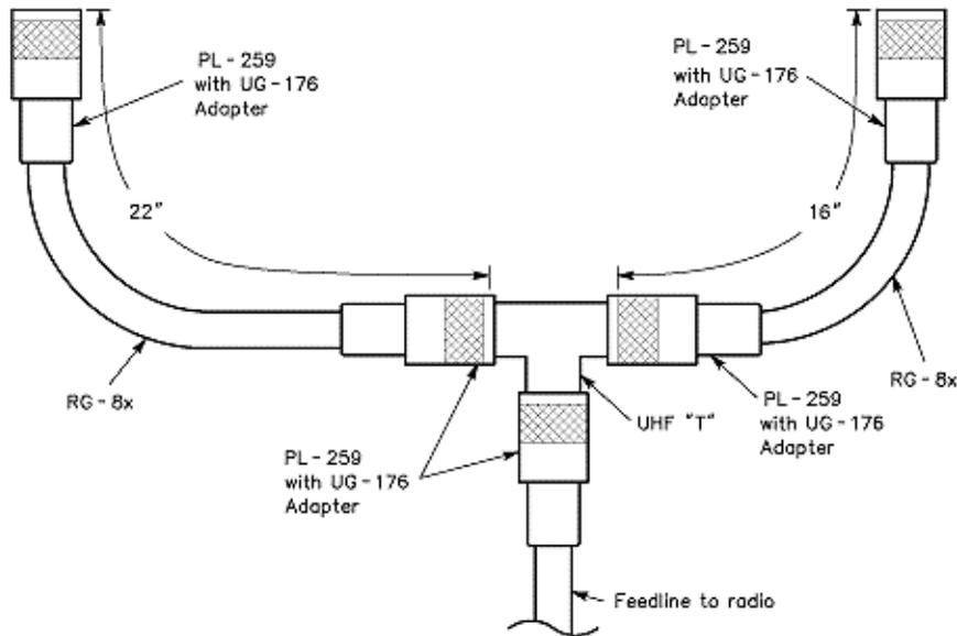
**Figure 4—The phasing harness. The lengths of the individual phasing lines are critical and should be as precise as possible. The direction of radiation is toward the antenna connected to the *longest* line.**
