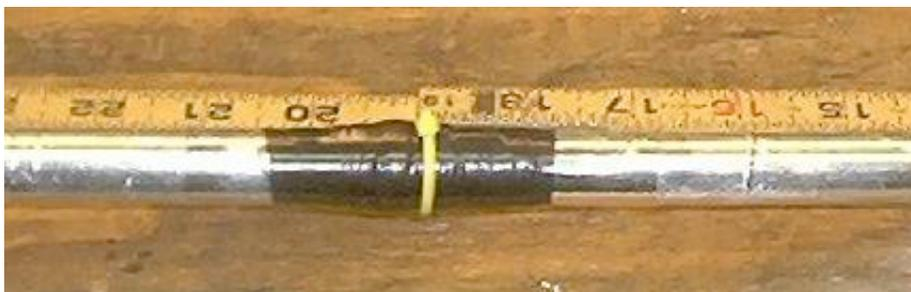
The antenna can be stuck down the back of the shirt, carried, or easily mounted on bicycles, etc. With a little more weatherproofing, it will make a fine dual-band base station antenna of moderate gain (2.2 dbi) and stealthy appearance (paint it the same color as your roof then clamp it to a vent pipe).
