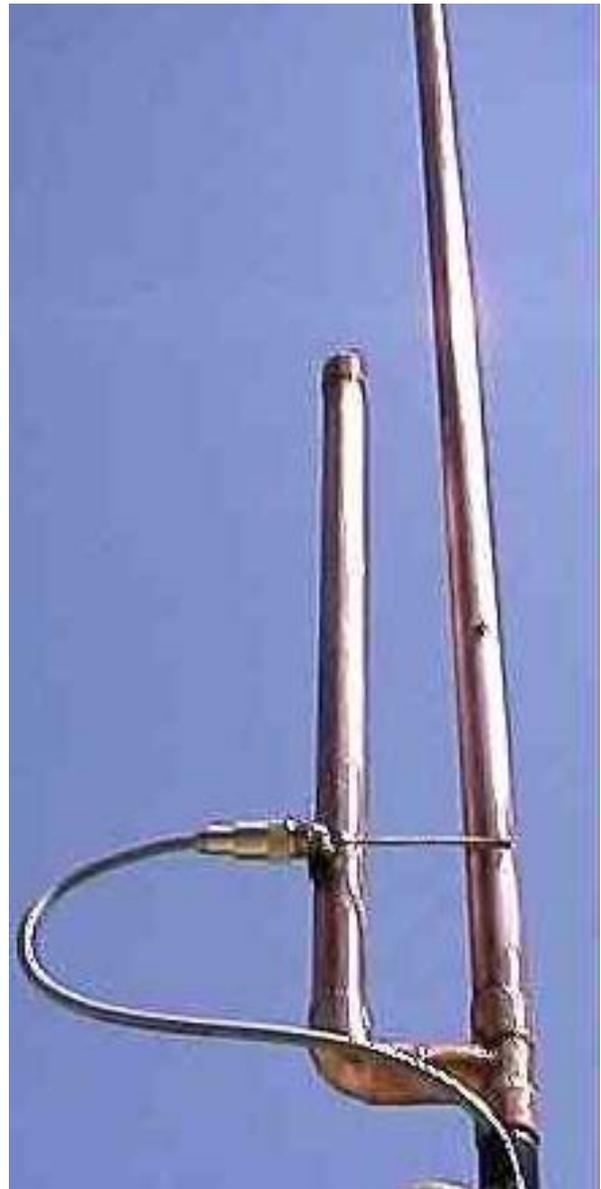
**NOTE:** Additional testing after creating this article I found that flipping the connections will improve 440 performance. Connect the coax center (brass rod) to the "short" element and attach the SO-239 to the long element for optimal performance.
